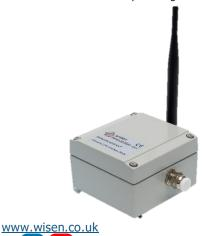
WiSenMeshWAN nodes communicate via bespoke encrypted mesh radio technology can be up to 1.5km from each other or the SmartGateway. The sensors mesh together and automatically form a network relaying data off each other (up to 6 sub mesh levels of data hop) and back to a central data hub called a SmartGateway which contains the data logging functions, radio mesh control systems and external communication to the WiSen cloud-based datacentre or local hosted system.
